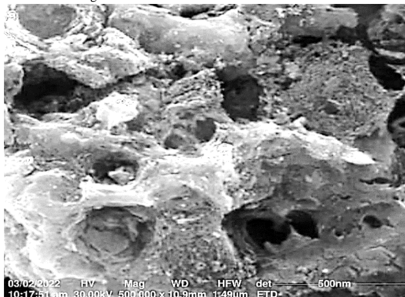
Figure 3: \text{VDZnCl}_2 adsorbent SEM micrograph
